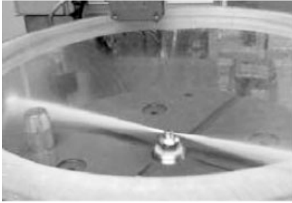
Fig. 7.18 (a) High-pressure water jet stream emerging from a nozzle [265].
