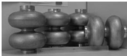
Fig. 6.28 (a) Several 3-cell hydroformed cavity sections for a 9-cell cavity [378]. (b) Several Nb-Cu hydroformed cavities [377] (courtesy of DESY).
