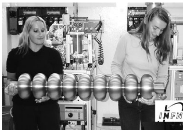
Fig. 6.32. The first 9-cell seamless cavity spun from a tube first made by flow turning [384] (courtesy of INFN).
