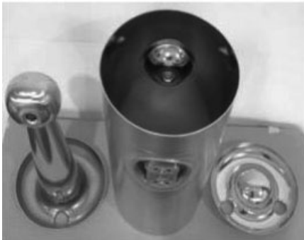
Fig. 6.22 Fabrication of (a) 115 MHz QWR for \beta=0.15 [375] and (b) a three-spoke niobium resonator [67] (courtesy of ANL).
