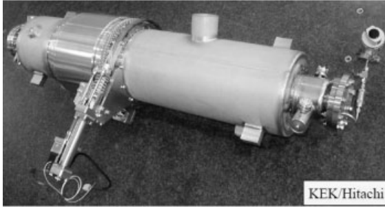
Fig. 10.8 Overview of the ball-screw tuner and helium vessel [577] (courtesy of KEK).
