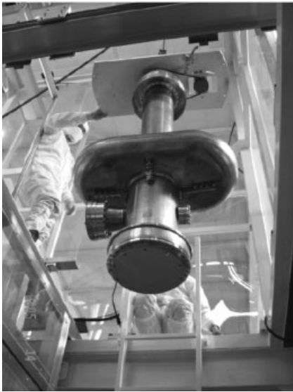
Fig. 11.11 (a) The crab-crossing scheme tilts bunches to provide head-on collisions. (b) High pressure water rinsing of the crab cavity. The cavity is 1 m by 0.5 m in cross-section. The cavity iris is reinforced by four ribs against stresses due to nonsymmetric cell shape [638, 639] (courtesy of KEK).
