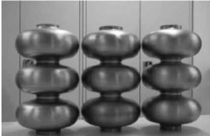
Fig. 6.28 (a) Several 3-cell hydroformed cavity sections for a 9-cell cavity [378]. (b) Several Nb-Cu hydroformed cavities [377] (courtesy of DESY).
