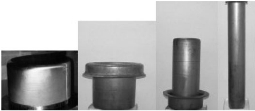
Fig. 6.34 Flow forming of a tube from a sheet in several stages [384] (courtesy of INFN).
