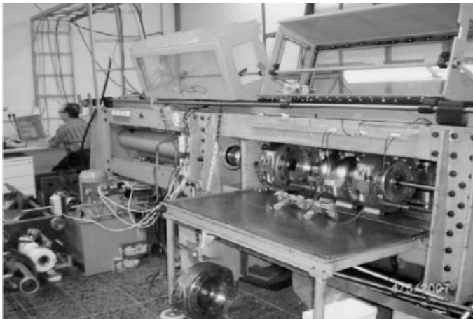
Fig. 6.26 Equipment for hydroforming used by DESY [182].
