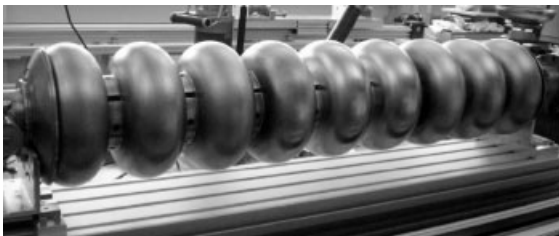
Fig. 6.29 A 9-cell hydroformed cavity by welding together three 3-cell sections [378] (courtesy of DESY).
