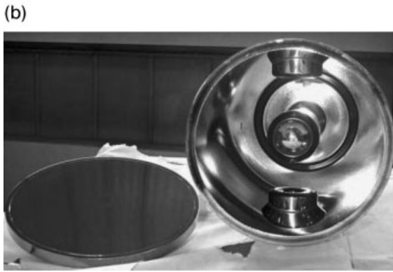
Fig. 11.32 (a) Evolution of ALPI energy with technology development [689]. (b) ALPI medium- \beta (0.11) Nb–Cu QWR [395, 689] (courtesy of INFN).
