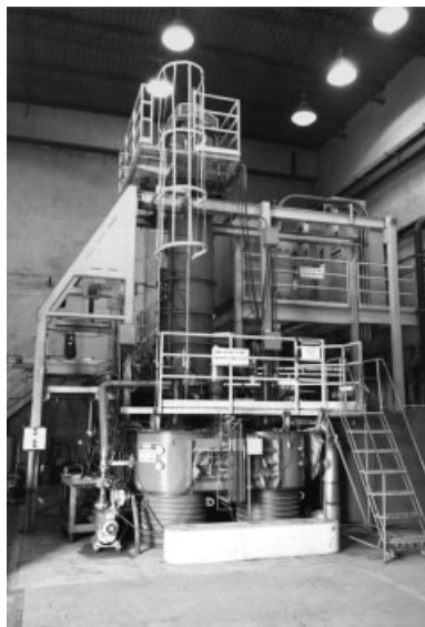
Fig. 6.1 Electron beam melting furnace at Wah Chang in Albany, Oregon [358].
