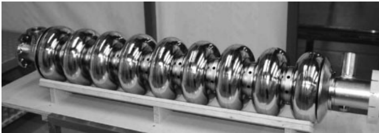
Fig. 6.17 A large grain 9-cell cavity fabricated at DESY [182].
