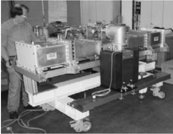
Fig. 8.30 CESR RF system waveguide window pair in high power test [463].
